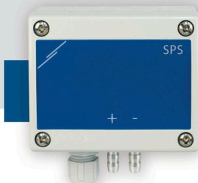
The SPS series are very compact differential pressure transmitters. They provide an analogue / modulating output and eight selectable measuring windows. The transmitters have an implemented state-of-the-art monolithic silicon pressure sensor and are equipped with Modbus RTU communication. These make the units suitable for a wide range of applications. The SPS piezoresistive transmitters are calibrated and temperature & pressure compensated. They feature a high degree of reliability and accuracy.
